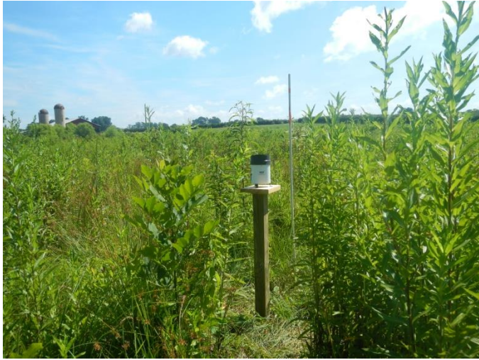
Rain gage installed (7/23/2013)
