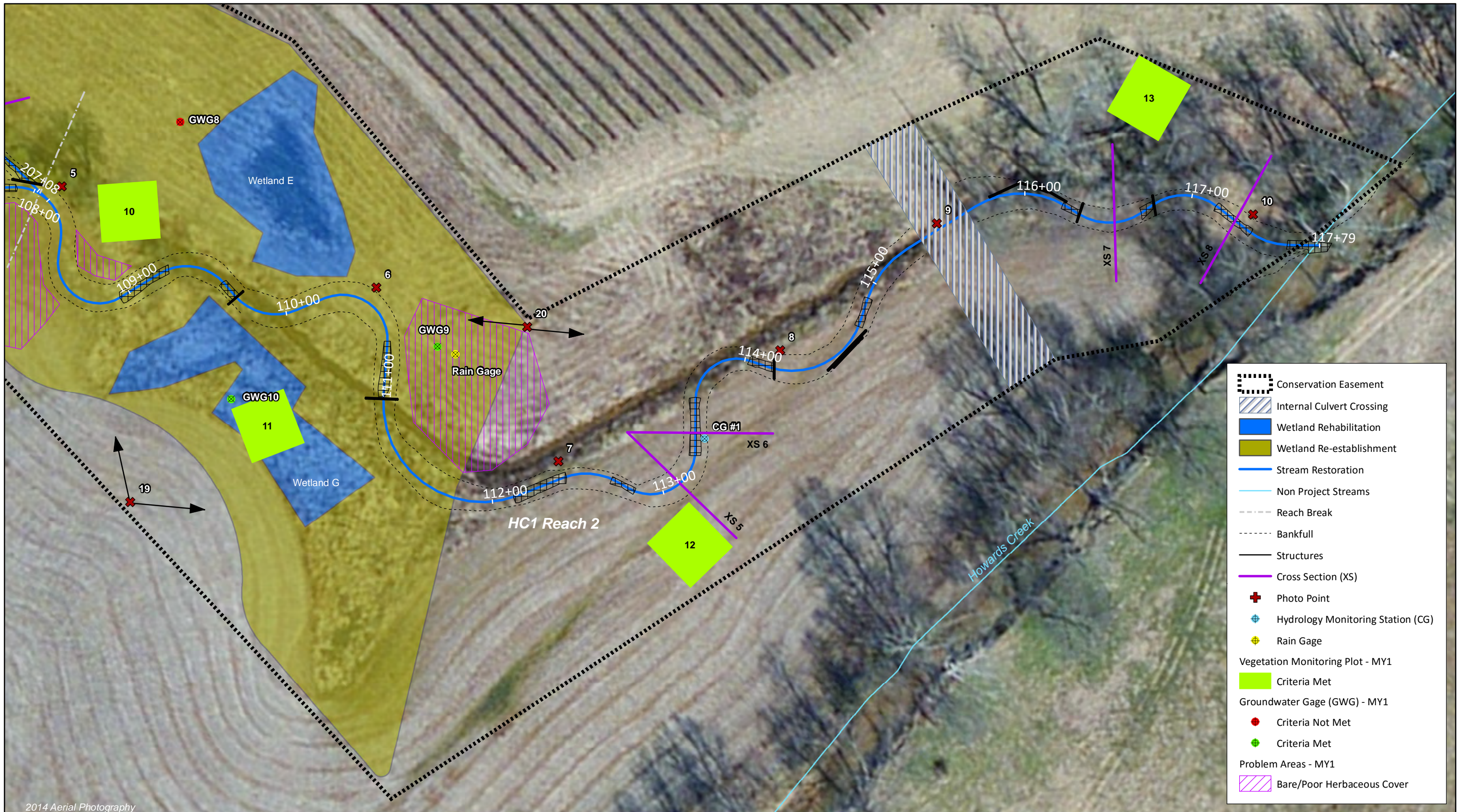
Figure 3.3 Integrated Current Condition Plan View (Sheet 3 of 3) Owl's Den Mitigation Site DMS Project No. 95808 Monitoring Year 1 - 2016 Lincoln County, NC
