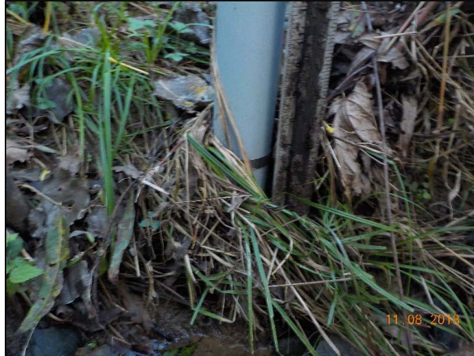
Wrack line @ Crest Gauge Thompson Branch – 0.67 ft. (Est. Date of Occurrence: 9/17/2018)
