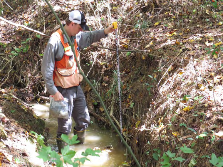
Reach R2- Bank erosion and incision (10/6/15)
