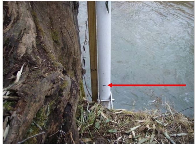
Bankfull elevation on crest gage noted with red arrow
