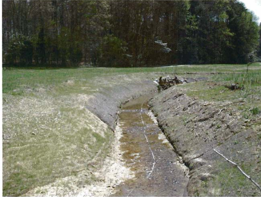
M9-US: View from Meander 9 looking upstream. Note the fiberglass tape is pulled across a riffle cross section near the center of the picture.
