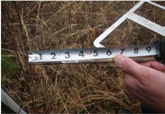
Photo 1. Crest gauge staff showing cork deposition at 5.87 inches above bankfull elevation, at the bottom of the gauge.
