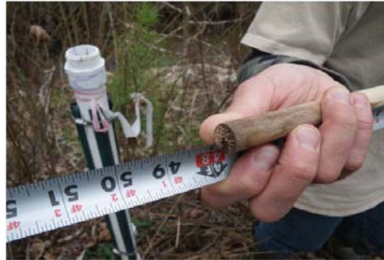
Photo 1. Crest gauge staff showing cork deposition on top of the staff indicating that flood waters were at or higher than 48 inches above
