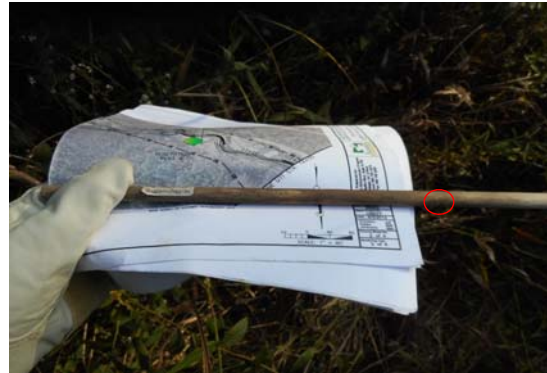
Photo 1. Crest gauge staff showing cork deposition in red circle at approximately 9 inches above bottom of staff, which is at bankfull, as measured against the 8.5 inch wide paper.
