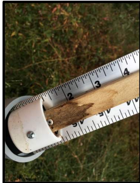
5.2 Crest Gauge UT 1 (10/5/2016)
