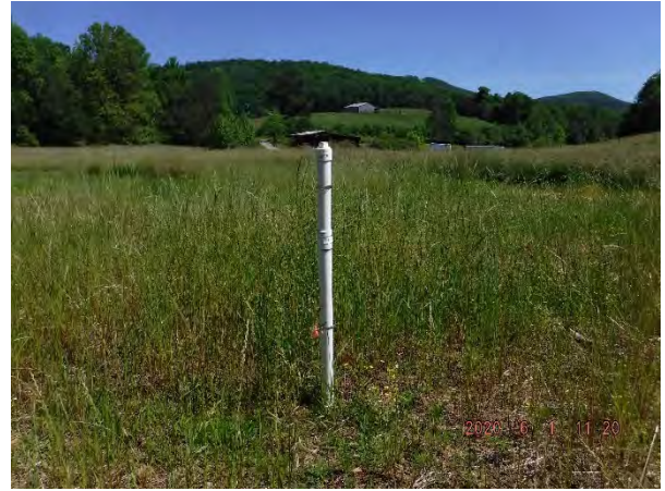
Crest Gauge #2, Reach 9, Station 40+10
