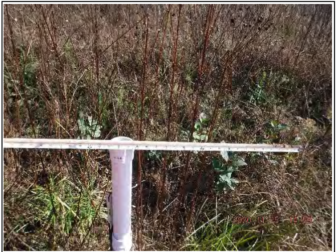
Crest Gauge 3 R4. BKF reading at 26" and 30." (November 5, 2020)
