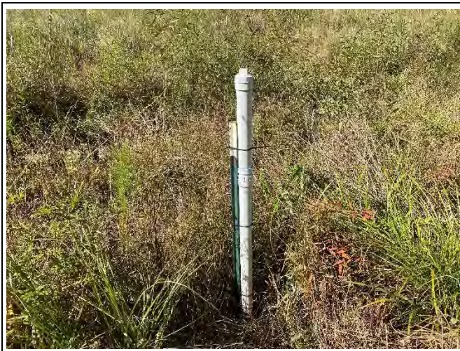
Crest Gauge 4 R6. (October 19, 2021)
