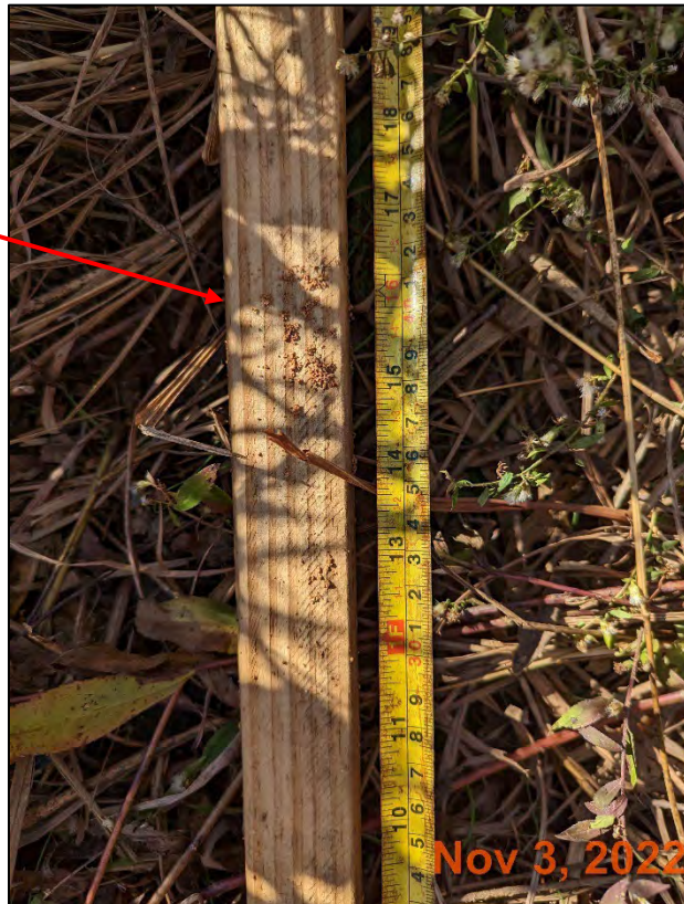
Photo #2 – Shadrick Creek Reach 3 Crest Gauge at 1.3 feet (Recorded ~bankfull)
