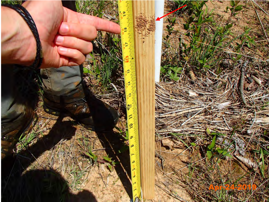
Photo #1 – Shadrick Creek Reach 1 Crest Gauge at 1.2 feet (Recorded bankfull 1.2 feet)
