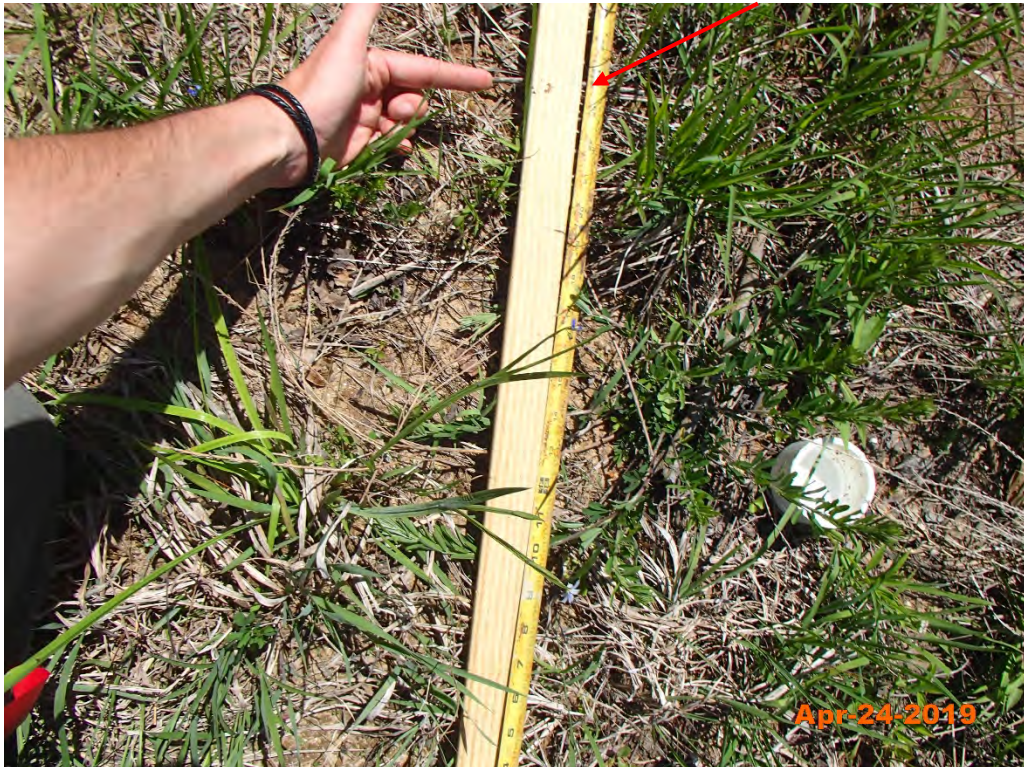
Photo #4 – Shadrick Creek Reach 3 Crest Gauge at 2.05 feet (Recorded bankfull 1.6 feet)
