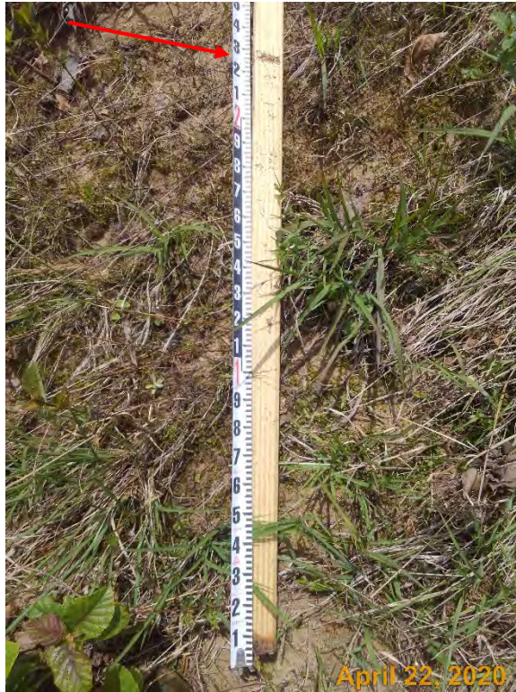
Photo #1 – Shadrick Creek Reach 1 Crest Gauge at 2.26 feet (Recorded bankfull 1.2 feet)
