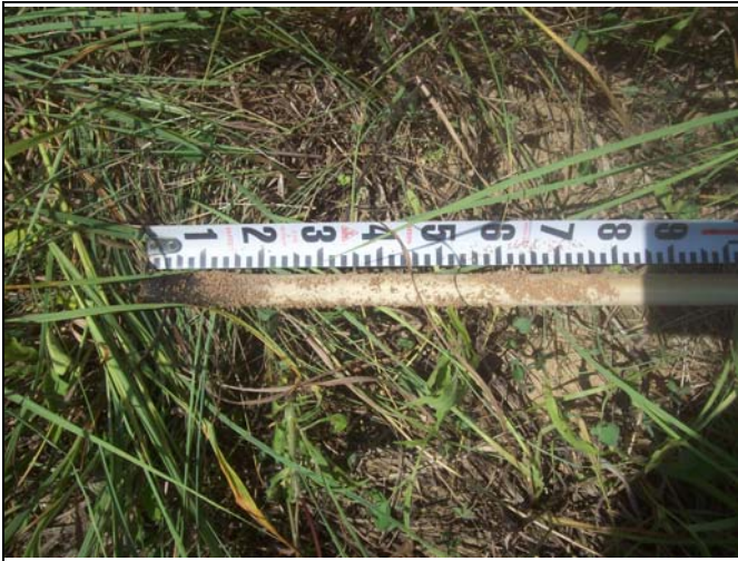
UT1 Crest Gauge - 0.79, June 28, 2010
