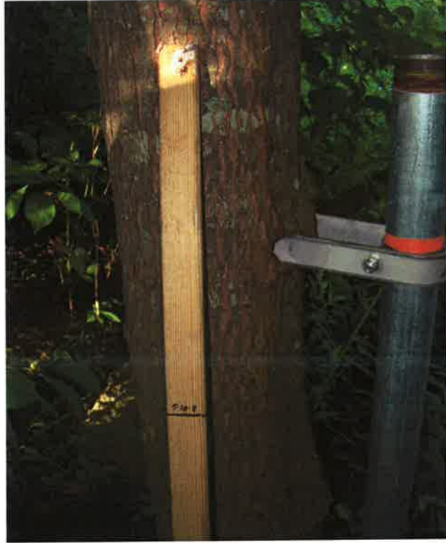
BF 5 Crest Gage on Silver Creek Mainstem (Year 5). (EMH&T, 5/20/11)
