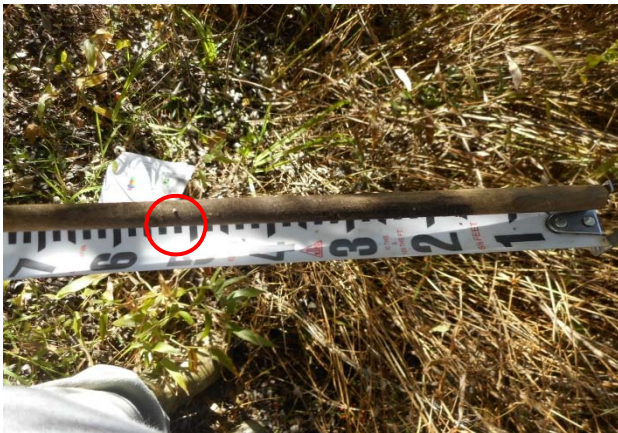
Photo1. Silver Creek crest gauge staff showing cork deposition in red circle at .52 ft above the bottom of the staff, which is at the bankfull elevation.
