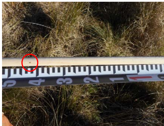
Photo 2. UT2 crest gauge staff showing cork deposition in red circle at 1.42 ft above the bottom of the staff, which is at the bankfull elevation.
