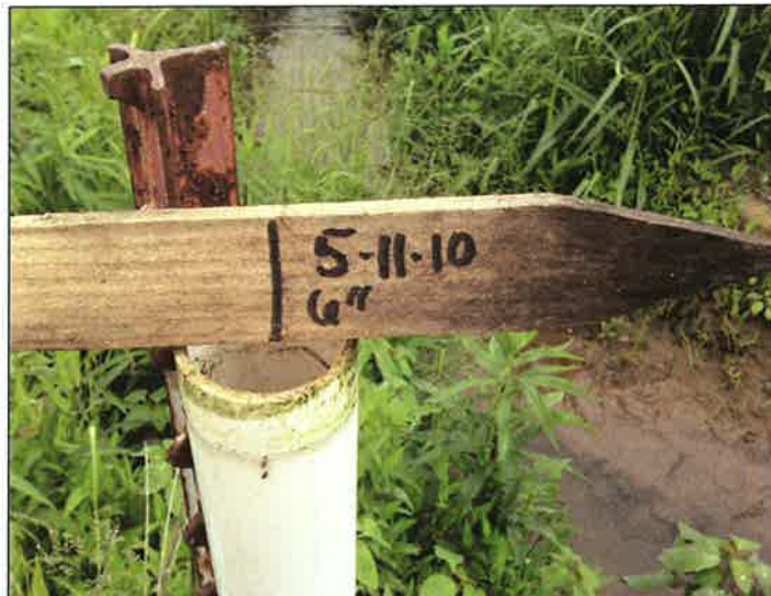
BF 16 Crest Gage on Tributary A2. (EMH&T, Inc. (documented, 5/11/10))
