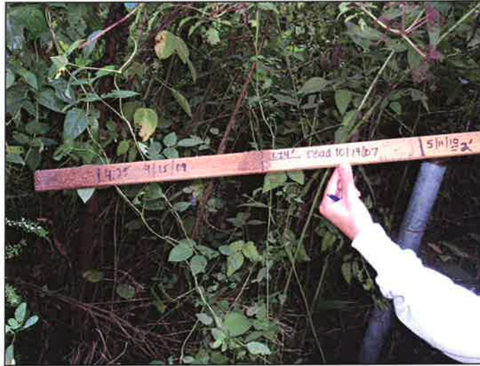
BF 13 Crest Gage at station 113+37 on Tributary A (upper). (EMH&T, Inc. (documented, 5/11/10))
