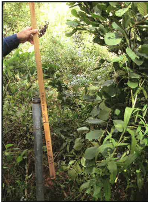
BF 8 Crest Gage on Tributary A (upper). (EMH&T, Inc. 9/21/09)
