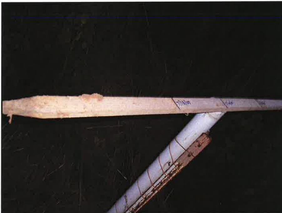
BF 2 Crest Gage at station 54+85 on Tributary A (lower). (EMH&T, Inc. 7/18/07)
