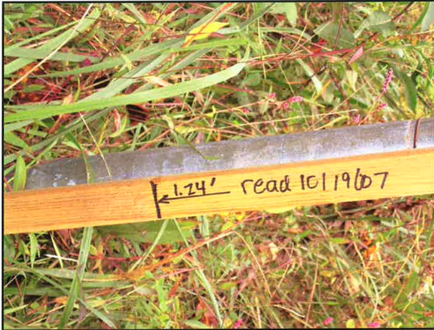
BF 3 Crest Gage at station 113+37 on Tributary A (upper). (EMH&T, Inc. 10/19/07)
