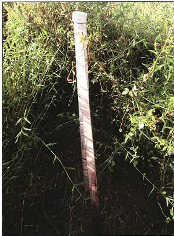
BF 14 Crest Gage at station 54+85 on Tributary A (lower). (EMH&T, Inc. (documented, 5/11/10))
