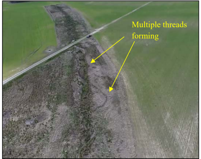
Photo 5. Development of multi thread channel system on T2
