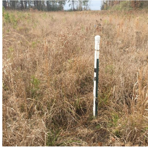
Flow Logger (UT2) – SCFL4, December 13, 2016 no flow present
