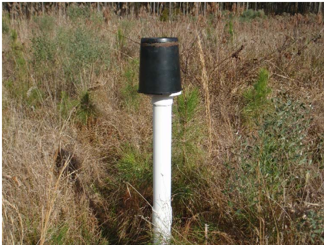
On-site rain gauge - adjacent to SCAW1
