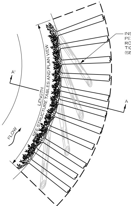
PLAN VIEW - 2 ROOTWAD INSTALLATION
