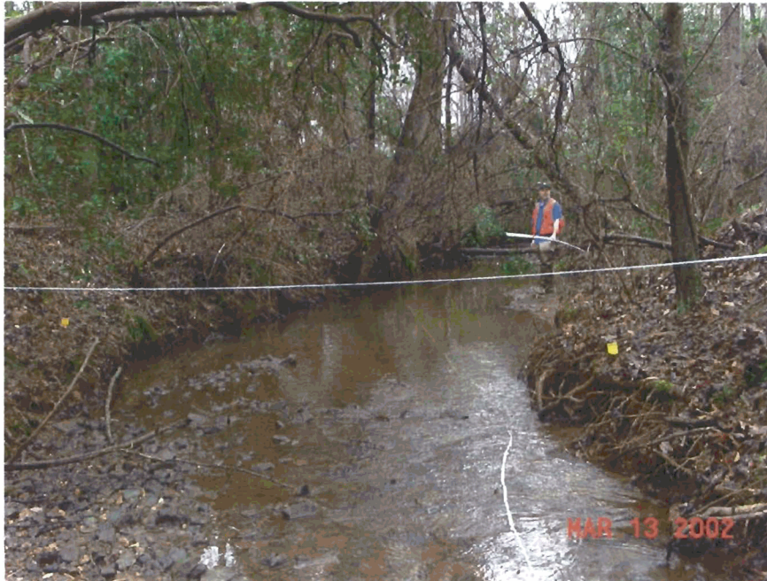
Photo 6: Looking downstream from the cross-section of the reference reach on Suck Creek approximately 300 feet downstream of Beulah Hill Church Road. The Rosgen stream type is B4.
