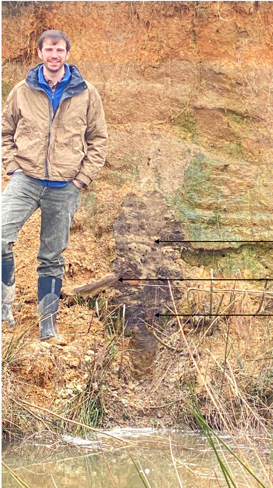
Photo 3.) UT-2 Failed Crossing – Historic floodplain elevation with historic tree roots visible at break between historic floodplain and fill material
