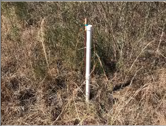
PP-31: Reach 2, Crest Gauge at Station 38+90
