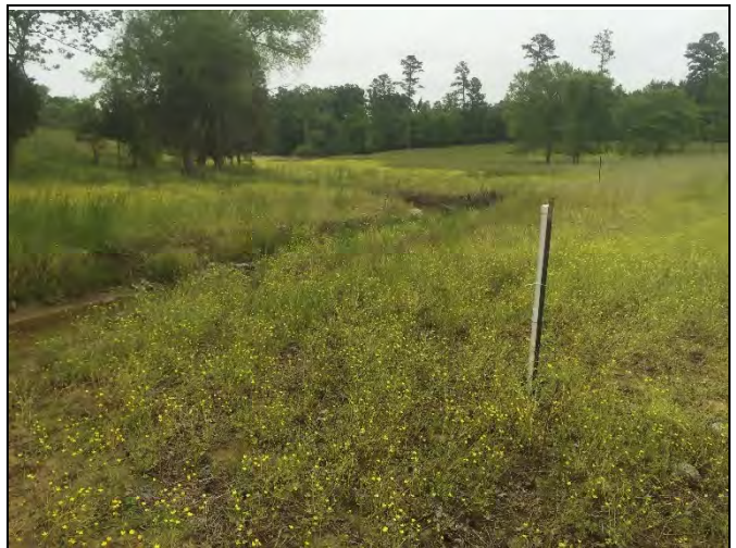
Crest Gauge on Reach R2 (photo: 5/18/16)
