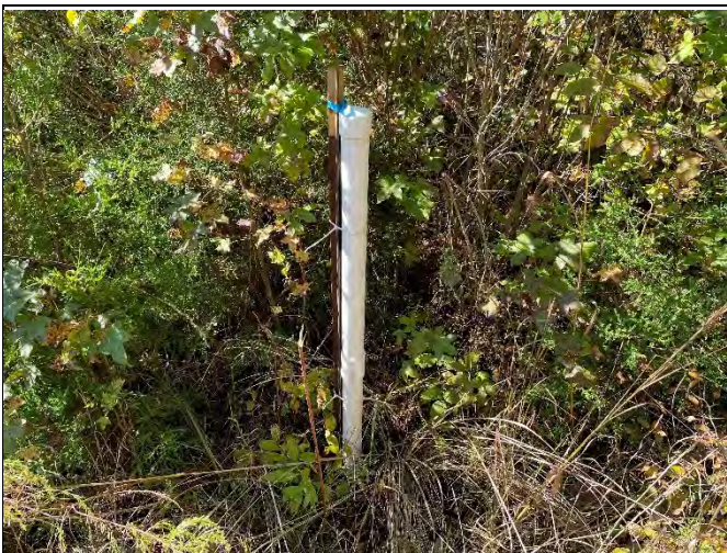
Crest Gauge on Reach R2 (photo: 10/19/22)
