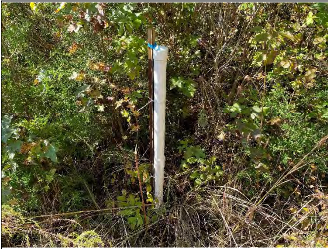
Crest Gauge on Reach R2 at Station 38+90 (photo from 10/19/22)
