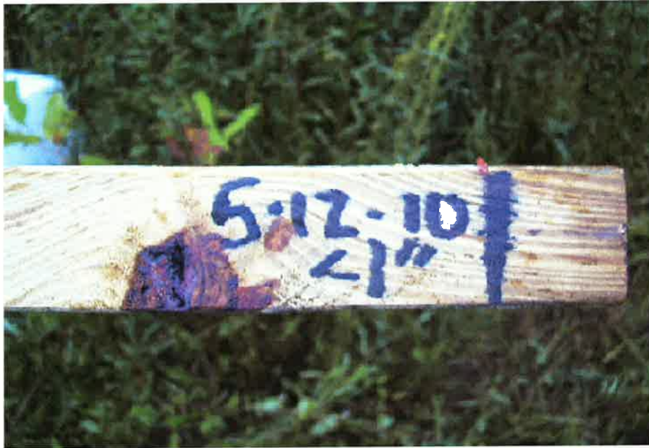
BF 1 Crest Gage at XS-6 on UT. (EMH&T, Inc. 5/12/10)
