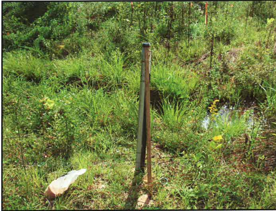
BF 1 Crest Gage at XS-6 on UT (Year 1). (EMH&T, 9/21/09)
