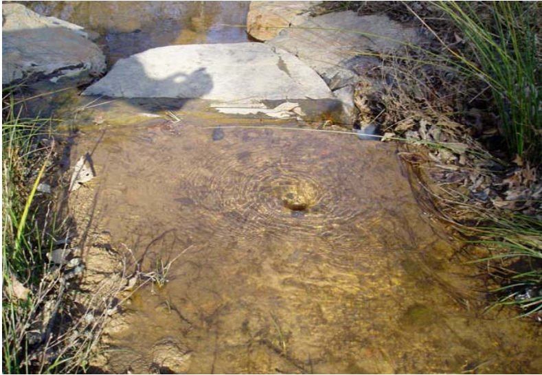
SP1. Piping and minor backcutting (hook/vane)
