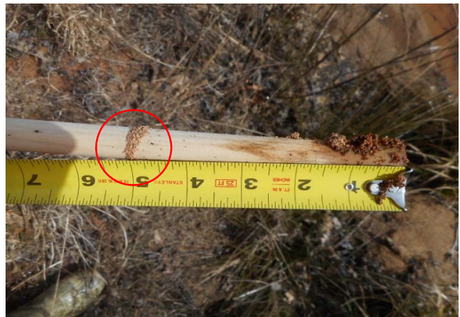
Photo 2. UT3 crest gauge staff showing cork deposition in red circle at 5.0 ft above the bottom of the staff, which is at the bankfull elevation.
