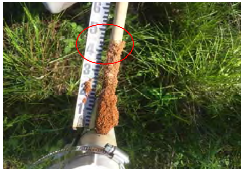
Photo 1. Silver Creek mainstem crest gauge staff showing cork deposition in red circle at 0.45' above the bottom of the staff, which is at the bankfull elevation. (5/2/2017)
