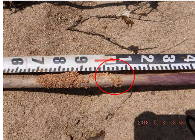
Photo 4. Silver Creek mainstem crest gauge staff showing cork deposition in red circle at 1.08' above the bottom of the staff, which is at the bankfull elevation (5/8/2018)
