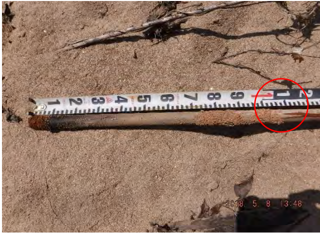
Photo 3. Silver Creek mainstem crest gauge staff showing cork deposition in red circle at 1.08' above the bottom of the staff, which is at the bankfull elevation (5/8/2018)
