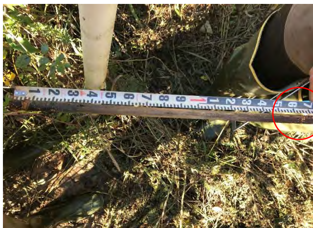
Photo 5. Silver Creek mainstem crest gauge staff showing cork deposition in red circle at 0.88' above the bottom of the staff, which is at the bankfull elevation (10/3/2018)
