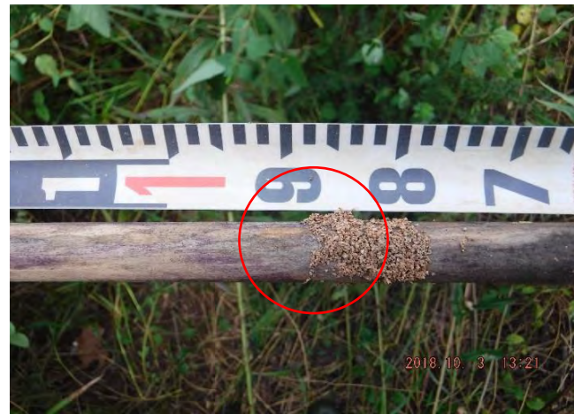
Photo 4. Silver Creek mainstem crest gauge staff showing cork deposition in red circle at 1.08' above the bottom of the staff, which is at the bankfull elevation (5/8/2018)
