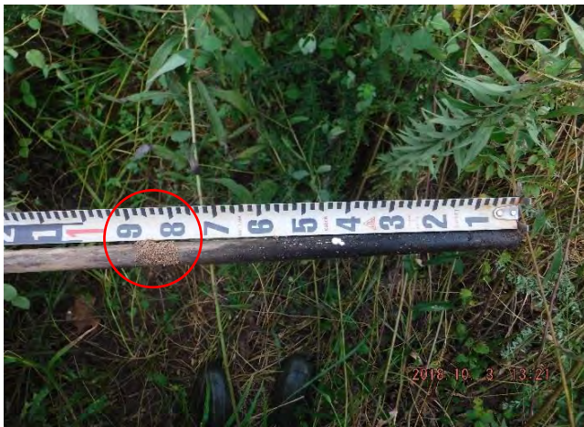
Photo 3. Silver Creek mainstem crest gauge staff showing cork deposition in red circle at 1.08' above the bottom of the staff, which is at the bankfull elevation (5/8/2018)
