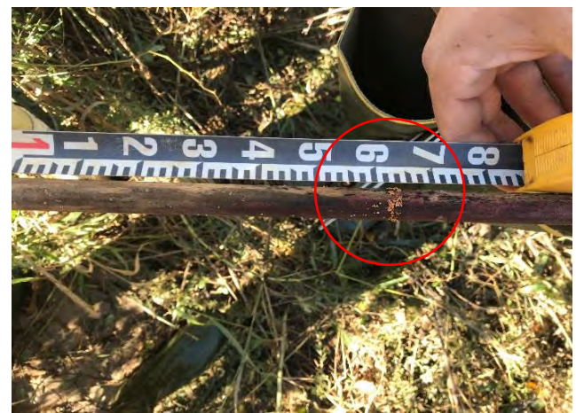
Photo 6. Silver Creek mainstem crest gauge staff showing cork deposition in red circle at 0.88' above the bottom of the staff, which is at the bankfull elevation (10/3/2018)
