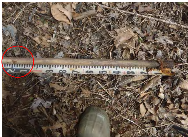
Photo 1. Silver Creek mainstem crest gauge staff showing cork deposition in red circle at 1.19' above the bottom of the staff, which is at the bankfull elevation (4/2/2018)
