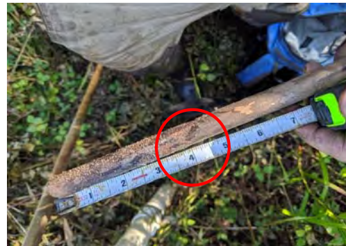
Photo 2. Silver Creek mainstem crest gauge staff showing cork deposition in red circle at 4.25" above the bottom of the staff, which is at the bankfull elevation (9/4/2019)
