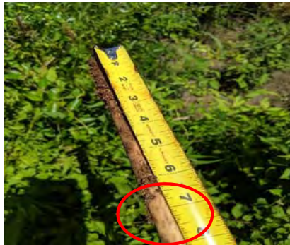
Photo 1. Silver Creek mainstem crest gauge staff showing cork deposition in red circle at 7.25" above the bottom of the staff, which is at the bankfull elevation (6/11/2019)
