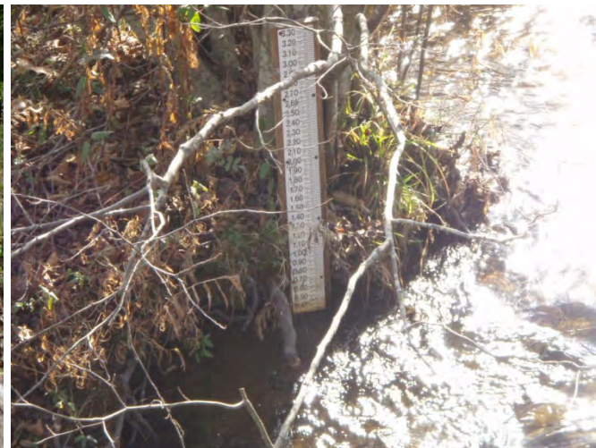
Stream gage plate, sta. 8+00, Mainstem 1 reach
