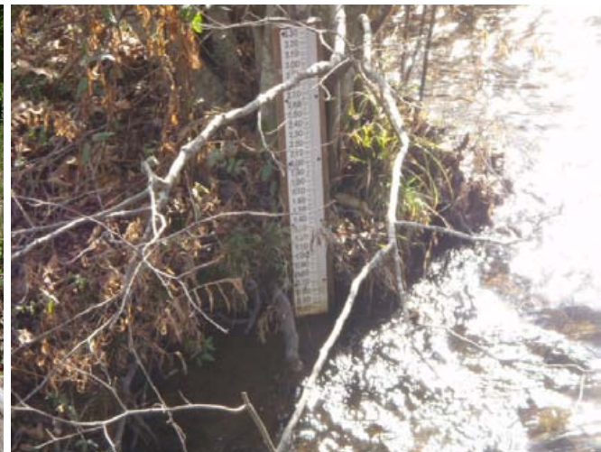
Stream gage plate, sta. 8+00, Mainstem 1 reach
