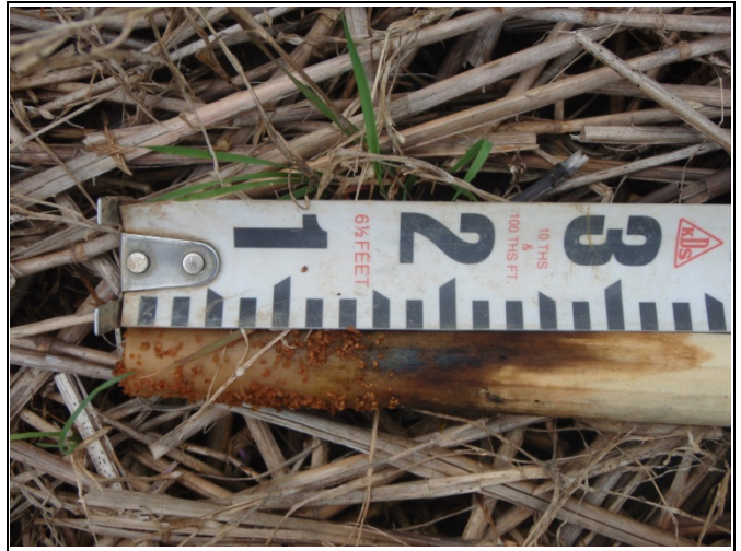
Crest gauge reading, 0.17 inches – October 16, 2013
