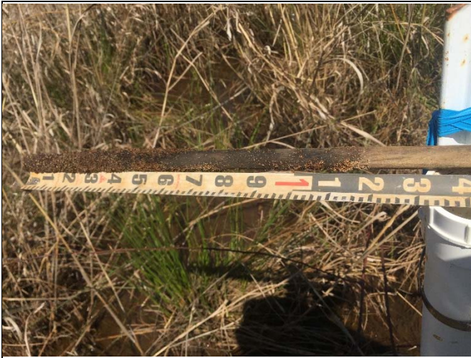
Crest gauge reading, 1.18 ft from 1/2/17 storm
