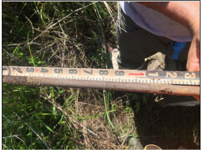
Crest gauge reading, 1.20 ft from 4/25/17 storm
