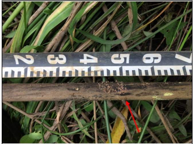
Crest gauge reading: 1.50 ft from 5/31/18 storm
