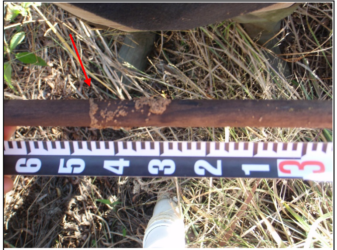
Crest gauge reading: 3.41 ft from 9/15/18 (Hurricane Florence)
