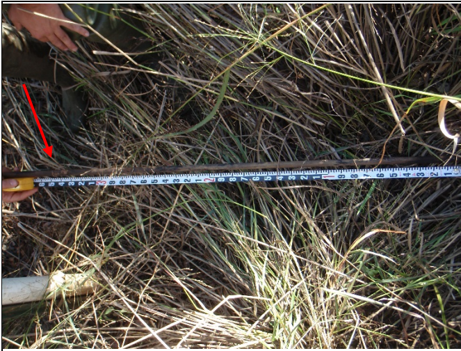
Crest gauge reading: 3.41 ft from 9/15/18 (Hurricane Florence)
