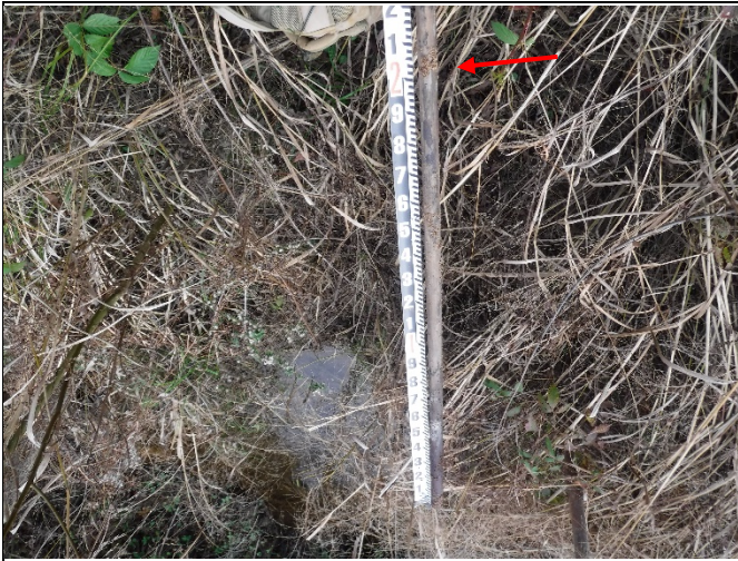
Crest gauge reading: 2.10 ft from 9/5/19 storm event
