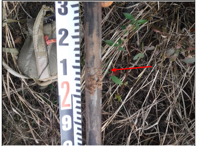
Close-up of crest gauge reading: 2.10 ft from 9/5/19 storm event
