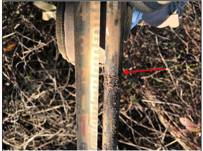
Close-up of crest gauge reading: 1.20 ft from 11/12/20 storm event
