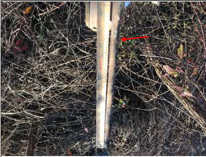
Crest gauge reading: 1.20 ft from 11/12/20 storm event (~4.9" rain)
