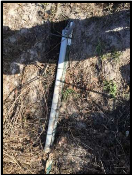
Figure 6.5 Damaged Crest Gauge 2/26/2016
