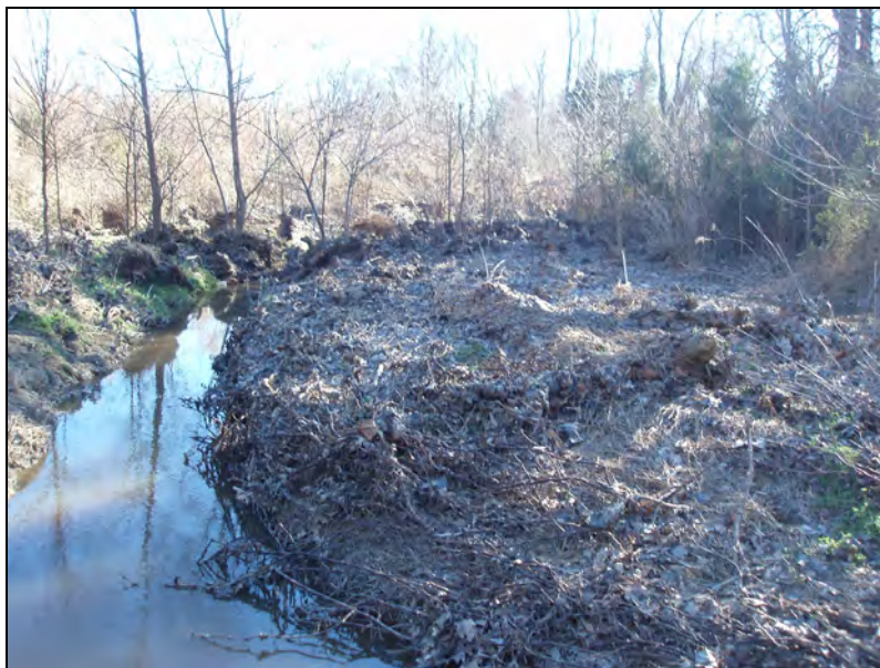
Photo 17. Bankfull indicators (wrack lines and flatten brush) - 1/3/2014
