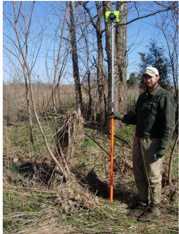
Photo 4: Bankfull flow event evidence (wrack line) at Station No. 10+00; Note foot of pole is resting at bankfull level; 3-16-2008.
