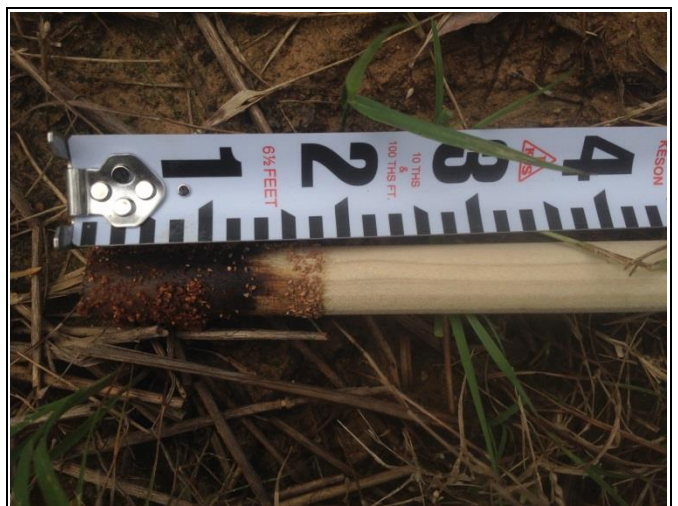
Reach R3 – Crest gauge reading, 0.18 inches, on October 1, 2014 (bankfull event ~July 16, 2014)
