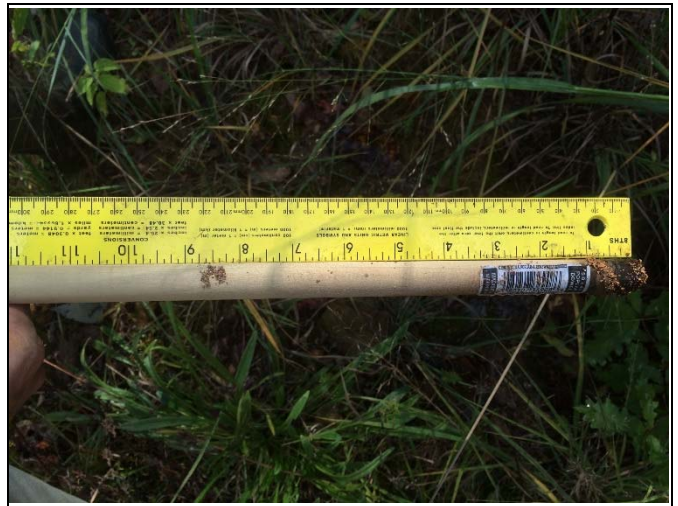
Reach R3 – Crest Gauge 2, 0.79 feet. October 13, 2015
