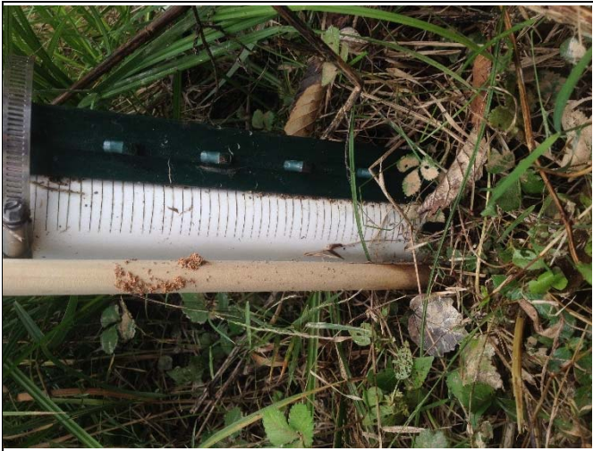
Reach R5 – Crest Gauge 1, 0.62 feet. October 13, 2015
