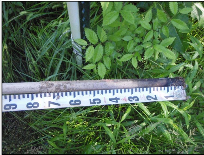
Reach R5: Crest Gauge #1, 0.76 feet on May 3, 2017
