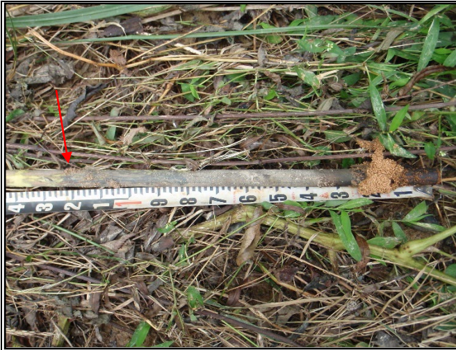
Reach R5: Crest Gauge #1, 1.22 feet on 9/24/18
