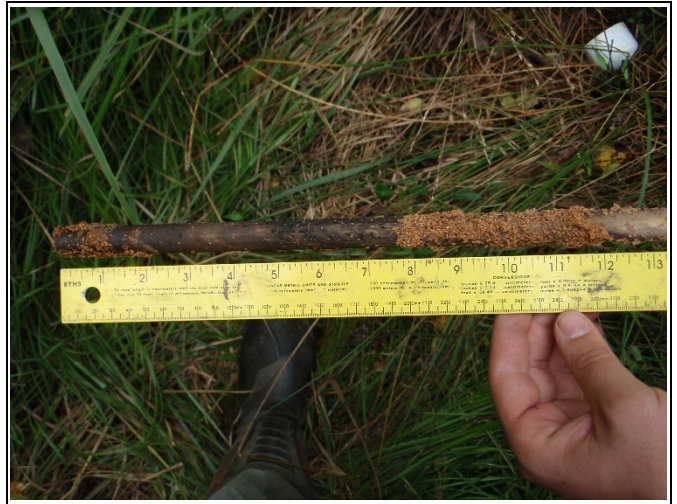
Reach R3: Crest Gauge #2, 1.08 feet on 9/24/18
