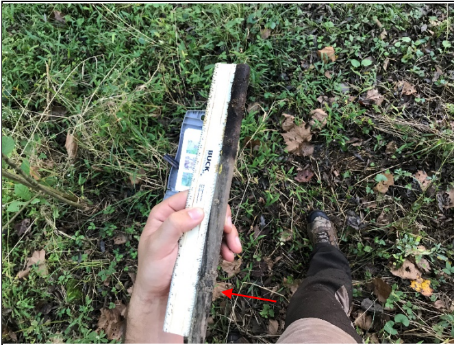
Reach R5: Crest Gauge #1, 0.83 feet on 6/6/19
