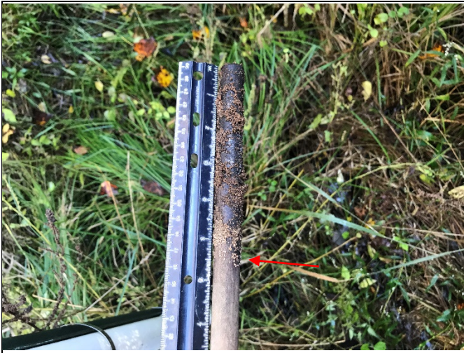
Reach R3: Crest Gauge #2, 0.46 feet on 6/6/19
