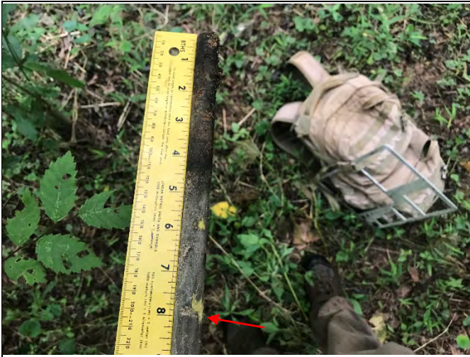
Reach R3: Crest Gauge #2, 0.67 feet on 8/28/2020 (after 2.47" storm event on 8/4 and 8/5)
