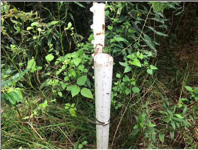
Reach R5: Crest Gauge #1 (ant colony destroyed cork indicators – has been cleaned and restored)
