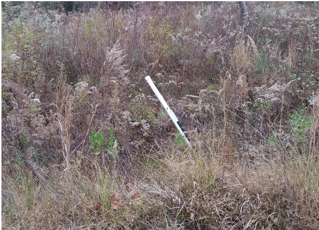
Crest Gauge (Main East) Leaning Over Following Bankfull Event
